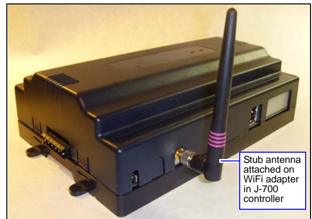
Figure 22 RP-SMA stub antenna on controller.
