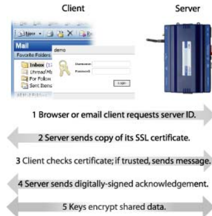
Figure 4-21 How SSL works
